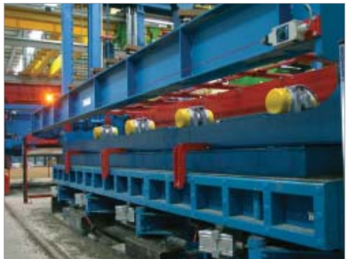
Compaction using load vibration
